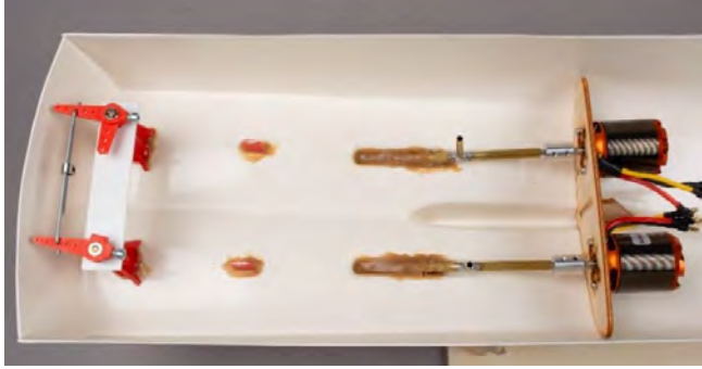
Fig.: Drive with Brushl. Max Marine P365 motors
