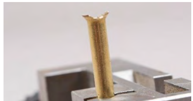
Fig.: Lubricating tube 3.3 round filed for soldering
