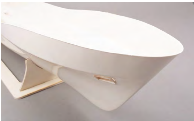
Fig.: Fitting the anchor pocket
