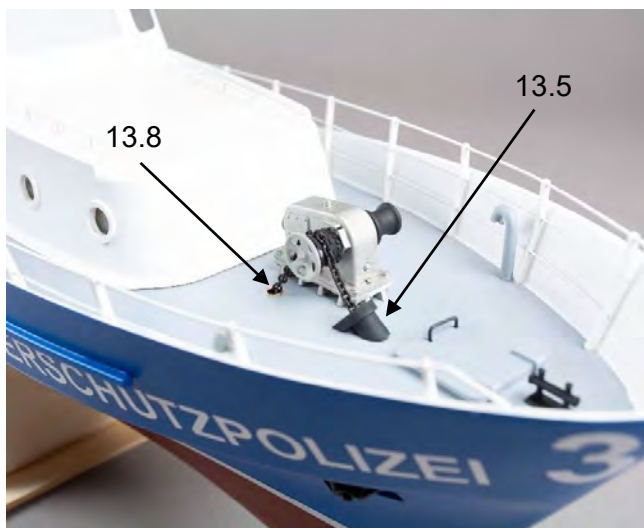
Fig.: Bow with anchor winch and hatch
