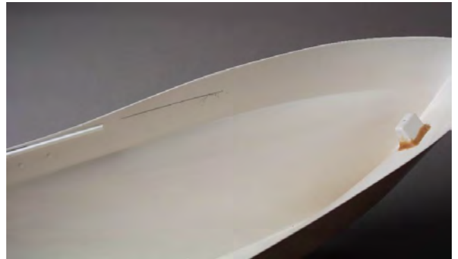
Fig.: Deck support rail at the bow
