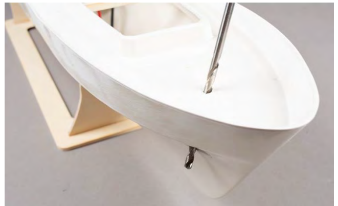
Fig.: Hole for anchor downpipe
